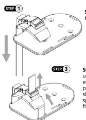
**Step 1:** Thread the toe strap webbing through the front slot of the foot plate.
