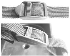
**NOTE:** The ladder buckle will need to be tightened against the shoe holder at the end of the adjustment process. Ensure that the length of strap remaining after the final adjustment is between the ladder buckle and the siderelease buckle and not between the ladder buckle and the body of the shoe holder. *Failing to move the buckle to the position below will result in slippage and loss of proper adjustment.*
