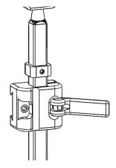
If adjustment to the HMO stop collar is necessary, use a 2mm hex key to loosen the collar's M5  $\times$  1  $\times$  5mm set screw. Slide the collar to the desired location, then secure the collar by tightening the screw.
