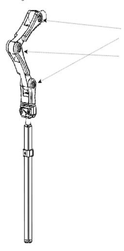
To make further adjustments to the final orientation of the headrest, loosen the three screws as shown in the image.
