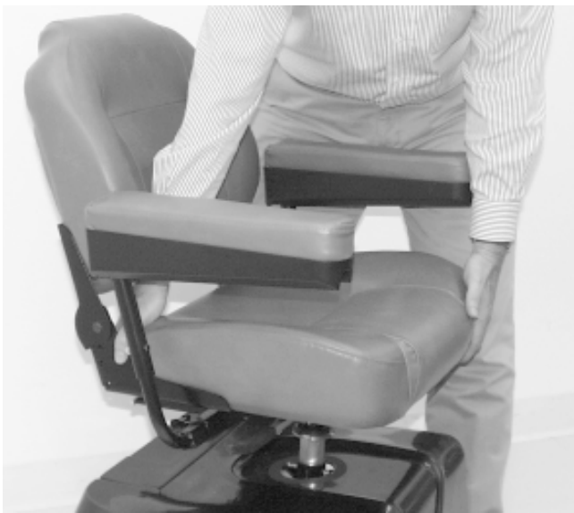
Figure 16. Removing the Seat
