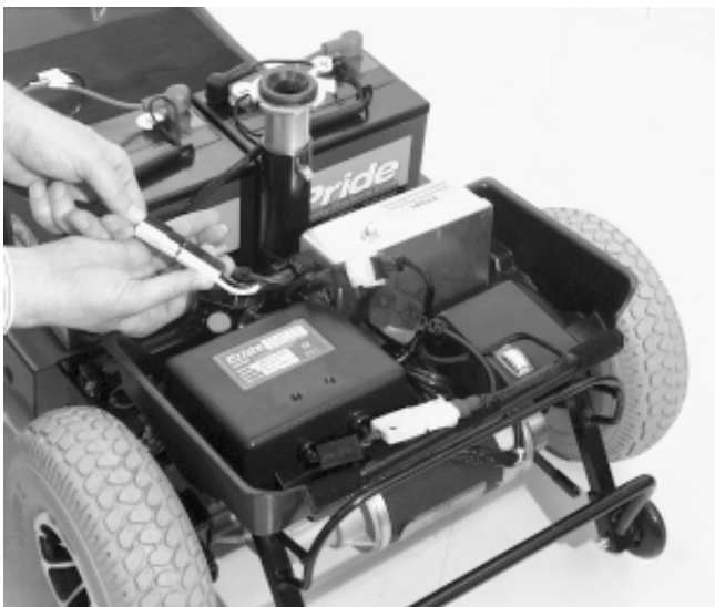
Figure 20. Unplugging the Battery Harnesses
