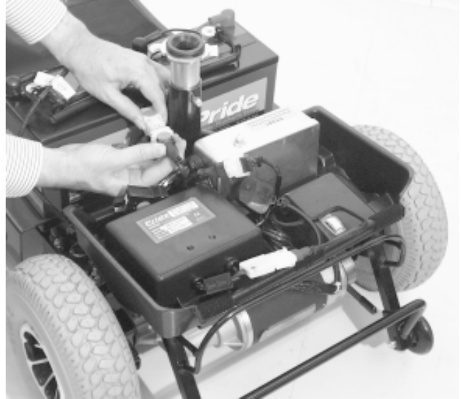
Figure 19. Unplugging the Front-to-Rear Connector
