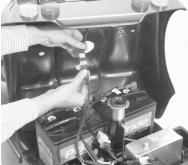
Figure 18. Unplugging the Rear Light Harness
