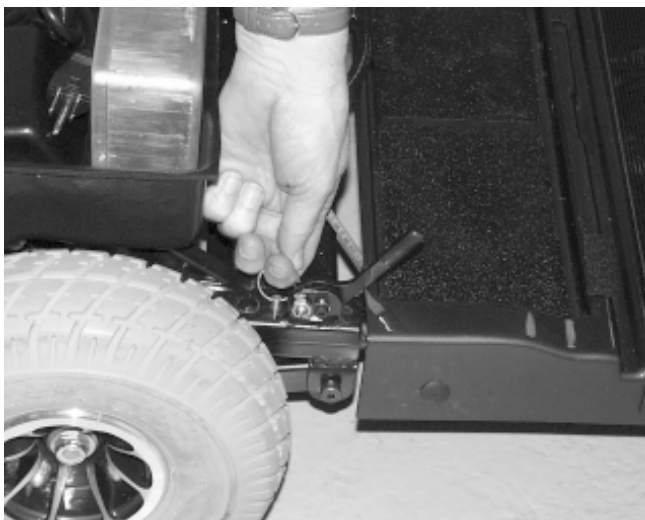
Figure 24. Removing Ball Detent Pins with Rings
