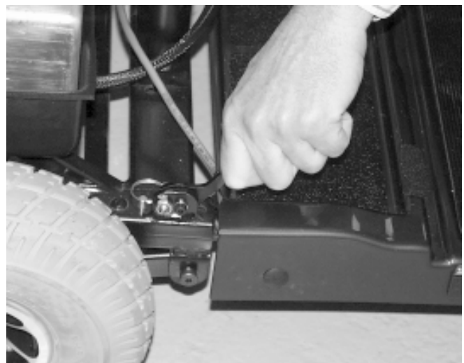
Figure 25. Lifting Up Locking Cam Levers
