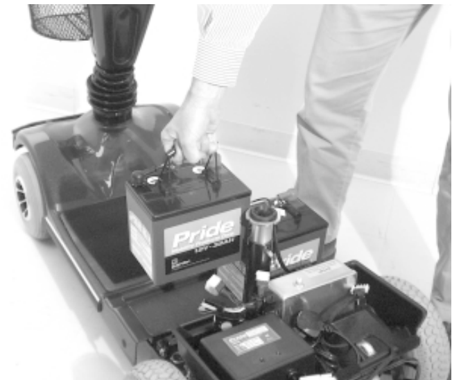
Figure 21. Lifting the Batteries
