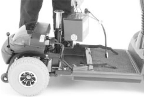
**FIGURE 22. BATTERY REMOVAL**
