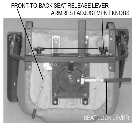
FIGURE 15. SEAT ADJUSTMENTS
