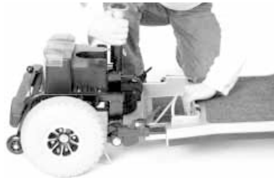
FIGURE 25. SEPARATING THE FRAME SECTIONS
