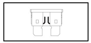
Figure 23A. Blown Fuse (Replace)
