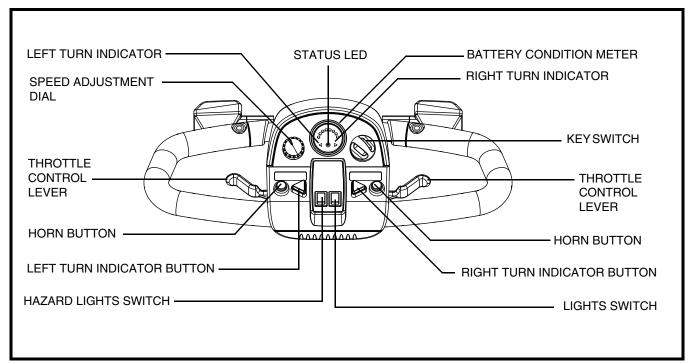
Figure 4. Tiller Console Components
