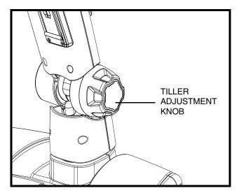
Figure 13. Tiller Adjustment
