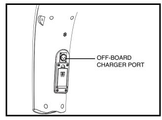
Figure 5. Off-board Charger Port (Tiller Mounted)
