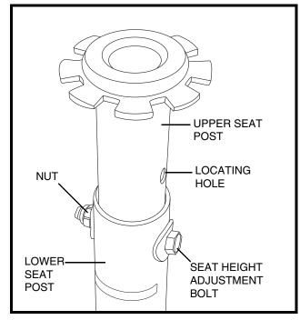
Figure 17. Seat Height Adjustment
