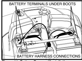
Figure 11. Battery Removal/Installation
