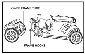
Figure 21. Frame Separation
