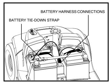
Figure 19. Harness Connections
