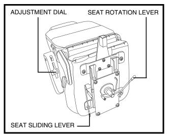
Figure 16. Seat Position Adjustments
