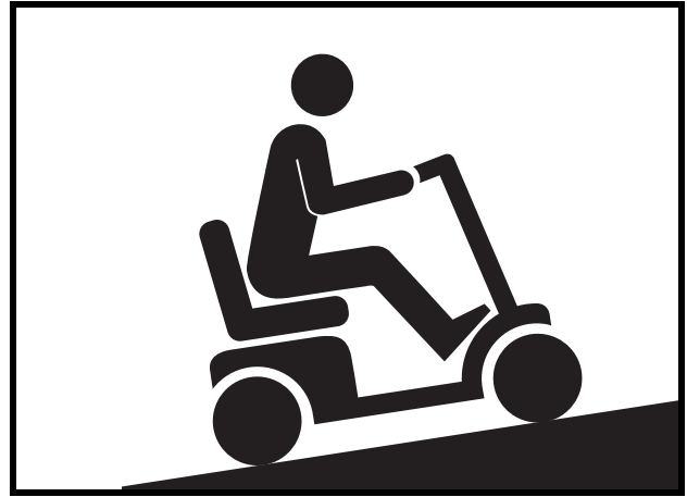
Figure 2. Increased Stability Driving Position
