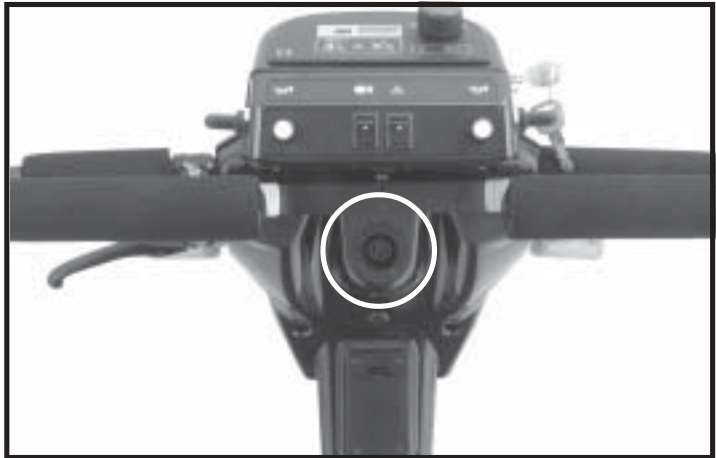
Figure 10. Charger Power Lead Receptacle
