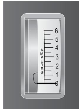
FIGURE 8A. AMMETRE INDICATES BATTERIES ARE FULLY CHARGED
