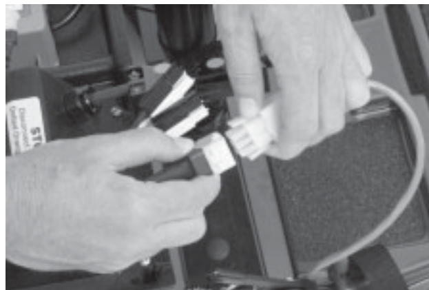
Figure 13. Unplug Front-to-rear Connector
