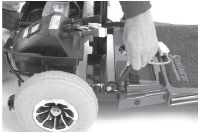
Figure 18. Push Cam Lock Levers Forward
