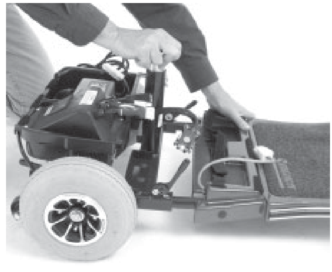
Figure 20. Separate Front and Rear Sections
