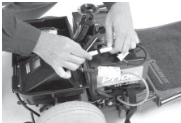
Figure 15. Unplug Battery Harnesses
