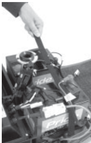
Figure 14. Unfasten Battery Tie-down Strap
