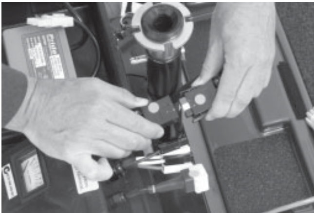
Figure 17. Disconnect Motor Harness Plug
