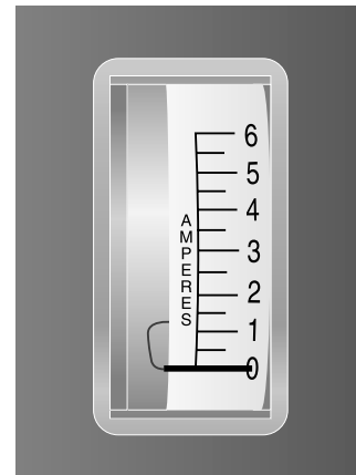
Figure 8. Ammeter Indicates Battery Is Fully Charged
