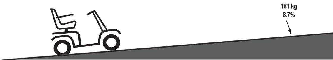
Figure 1. Maximum Recommended Incline Angle
