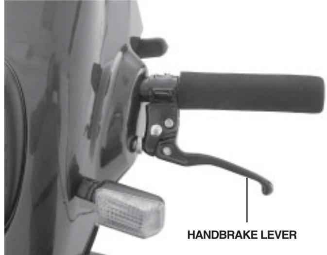
Figure 7. Handbrake Lever
