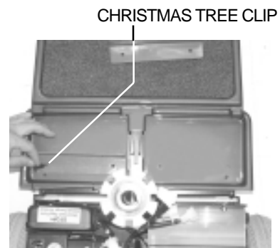
FIGURE 8A. INSTALLING THE CHRISTMAS TREE CLIPS
