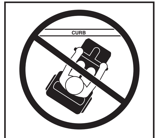
Figure 7. Incorrect Curb Approach
