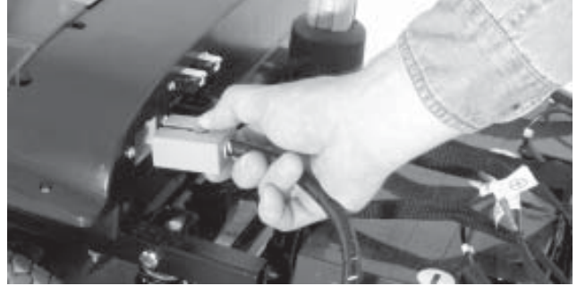
FIGURE 21. DISCONNECTING THE FRONT-TO-REAR HARNESS
