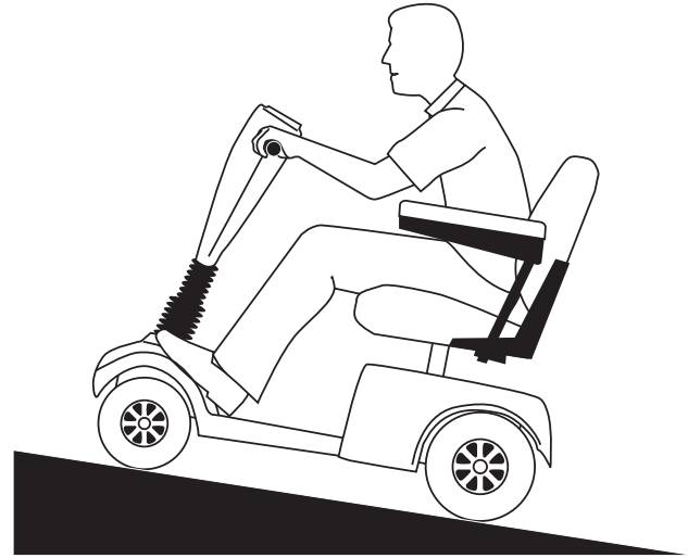
Figure 2A. Increased Stability Driving Position
