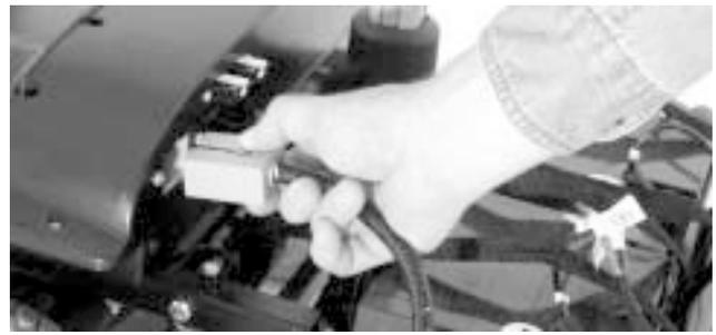
FIGURE 21. DÉBRANCHEMENT DU CÂBLE DE LA SECTION AVANT
