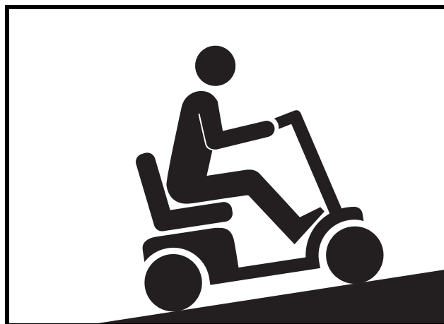
Figure 2. Increased Stability Driving Position
