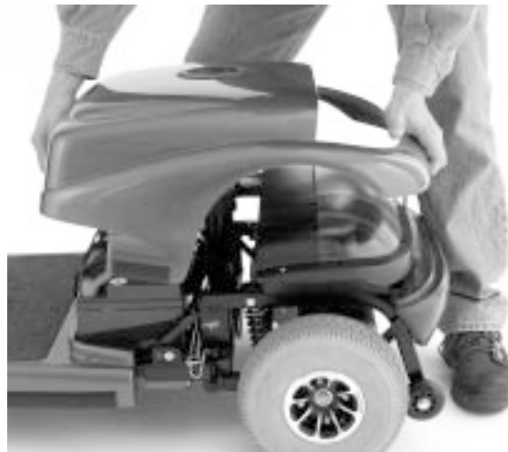
FIGURE 19. REAR SHROUD REMOVAL
