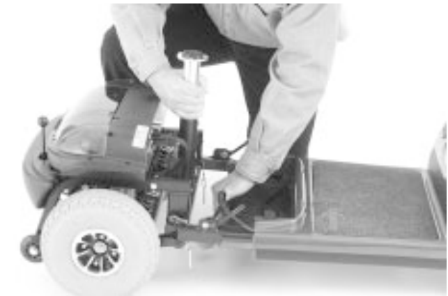
FIGURE 25. SEPARATING THE FRAME SECTIONS
