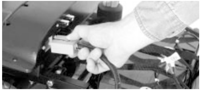
FIGURE 21. DISCONNECTING THE FRONT-TO-REAR CABLE
