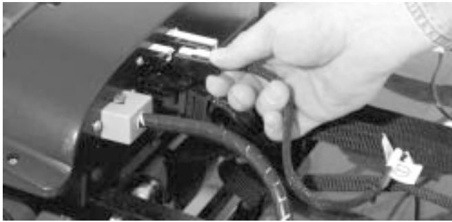
FIGURE 20. DISCONNECTING THE BATTERY HARNESES
