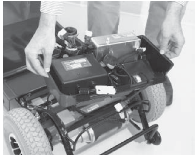
Figure 23. Lifting the Utility Tray
