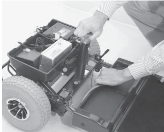
Figure 26. Separating the Frame Sections
