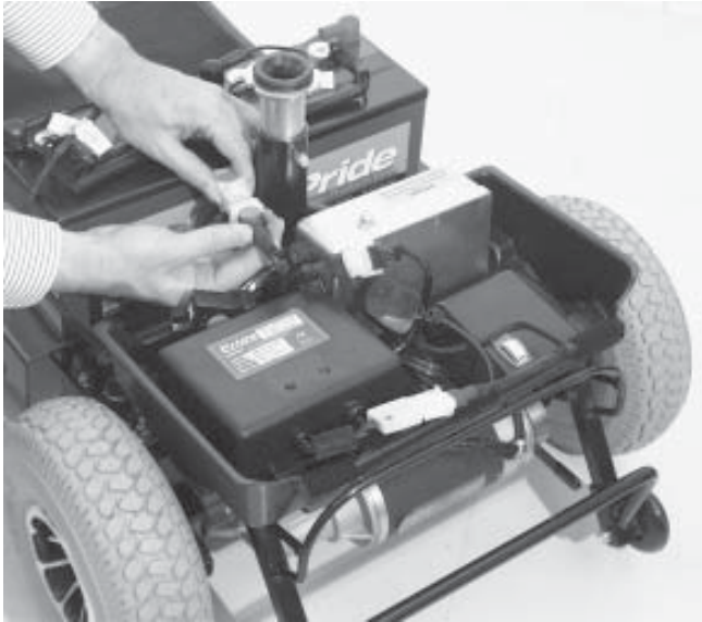
Figure 18. Unplugging the Rear Light Harness
