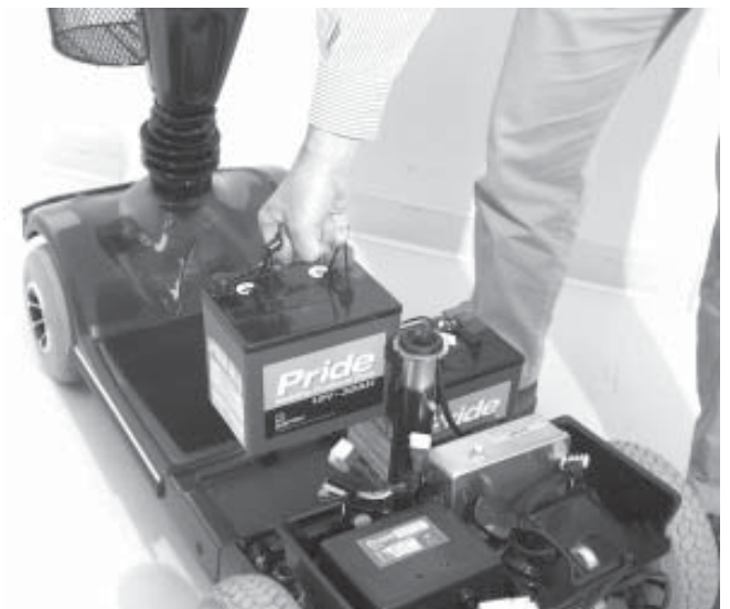
Figure 21. Lifting the Batteries
