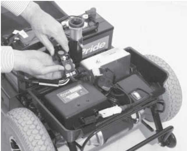
Figure 22. Disconnecting the Motor Harness
