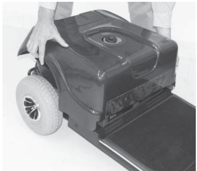
Figure 17. Removing the Shroud
