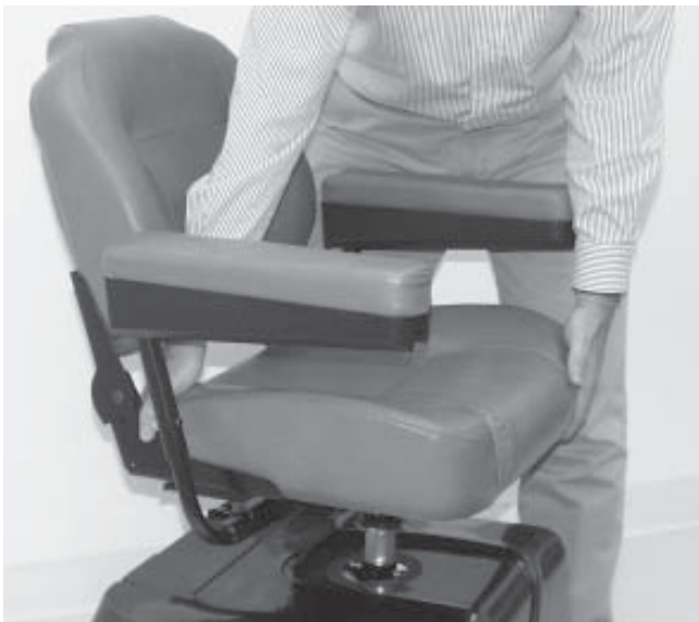
Figure 16. Removing the Seat
