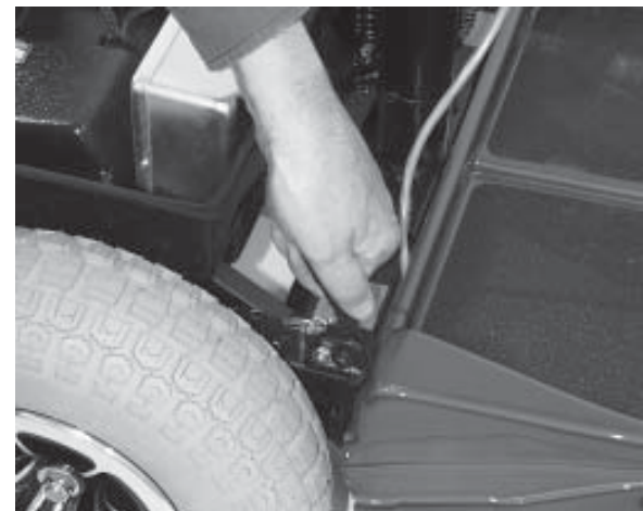
Figure 24. Lifting Up Locking Cam Levers
