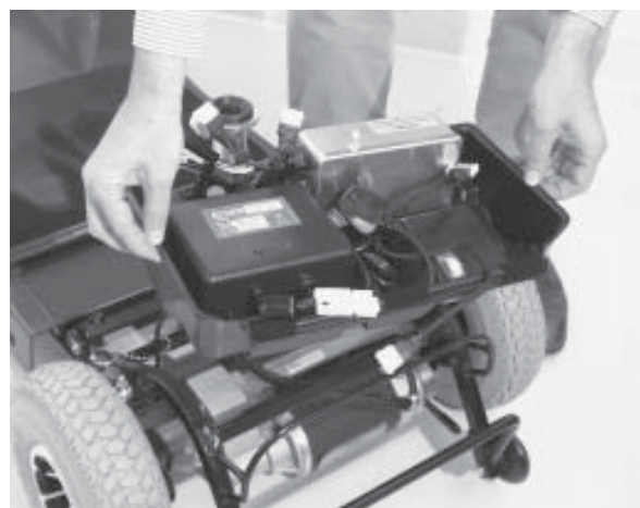
Figure 22. Lifting the Utility Tray
