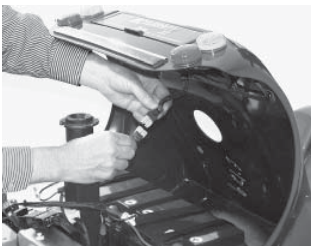
Figure 17. Disconnecting the Lighting Harness
