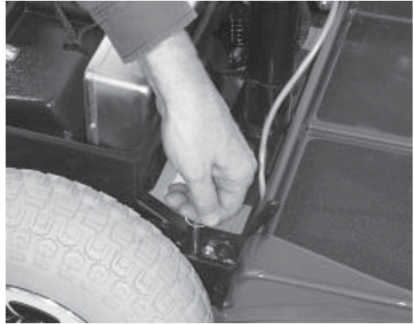
Figure 23. Removing Ball Detent Pins with Rings
