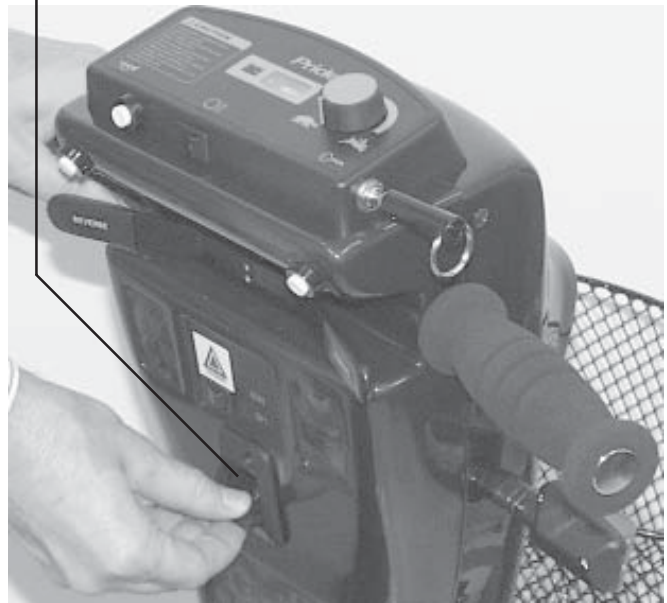
Figure 10. Tiller Angle Adjustment
