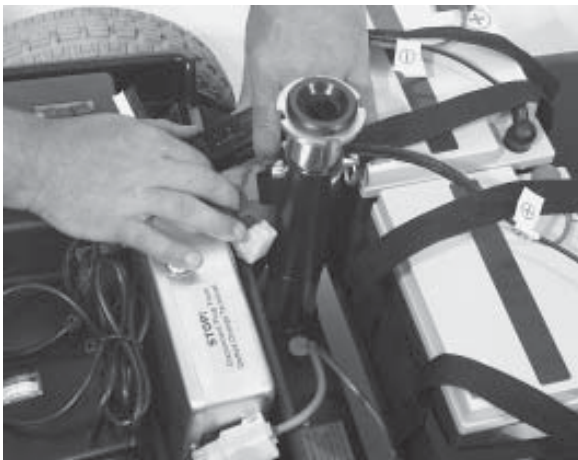
Figure 21. Disconnecting the Motor Harness
