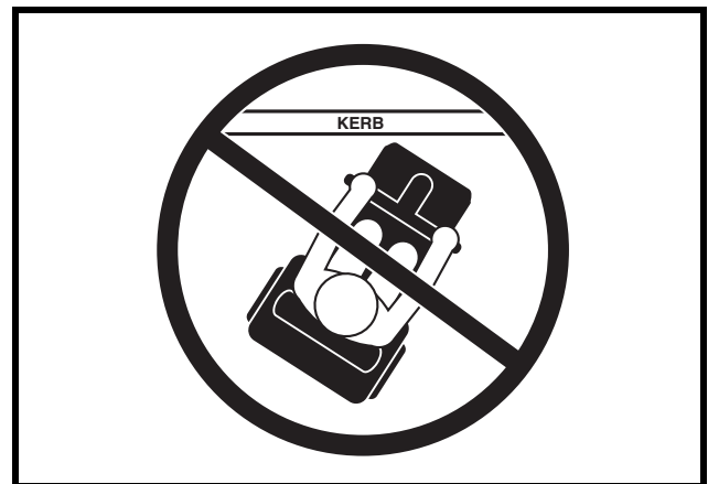
Figure 3A. Incorrect Kerb Approach
