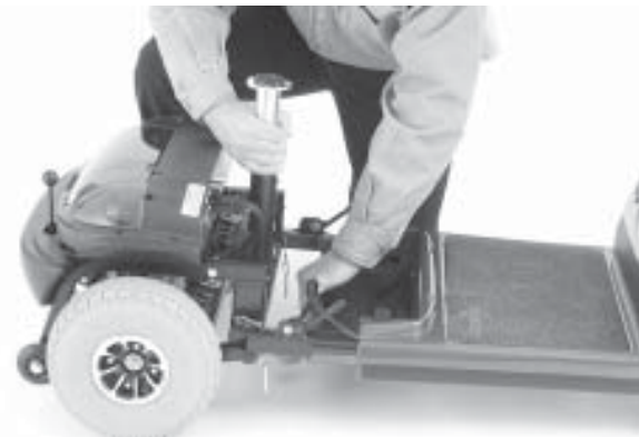
FIGURE 26. SEPARATING THE FRAME SECTIONS
