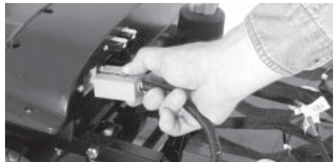
FIGURE 21. DISCONNECTING THE FRONT-TO-REAR HARNESS
