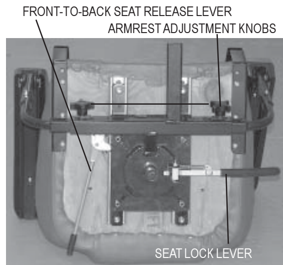
FIGURE 15. SEAT ADJUSTMENTS
