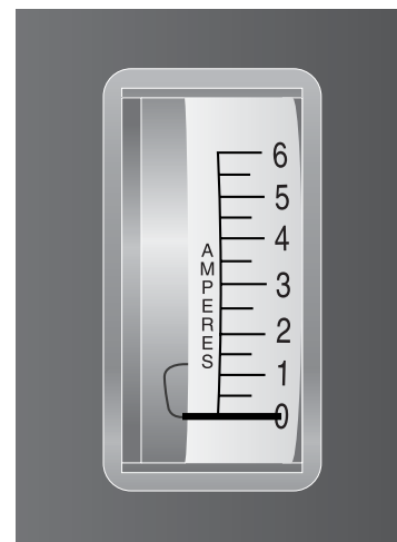
FIGURE 12. AMMETER INDICATES BATTERY IS FULLY CHARGED
