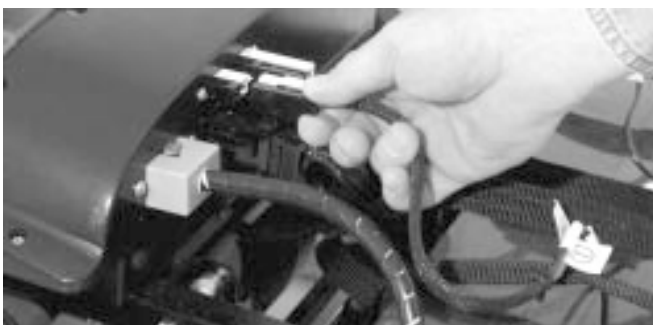
FIGURE 20. DISCONNECTING THE BATTERY HARNESSSES
