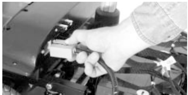
FIGURE 21. DISCONNECTING THE FRONT-TO-REAR HARNESS
