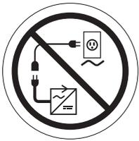
Prevent personal injury and equipment damage. Do not connect an extension lead to the AC/DC converter or the battery charger.
