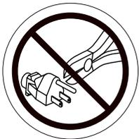
Removal of grounding prong can create electrical hazard. If necessary, properly install an approved 3-pronged adapter to an electrical outlet having 2-pronged plug access. Failure to heed could result in personal injury and/or property damage.
