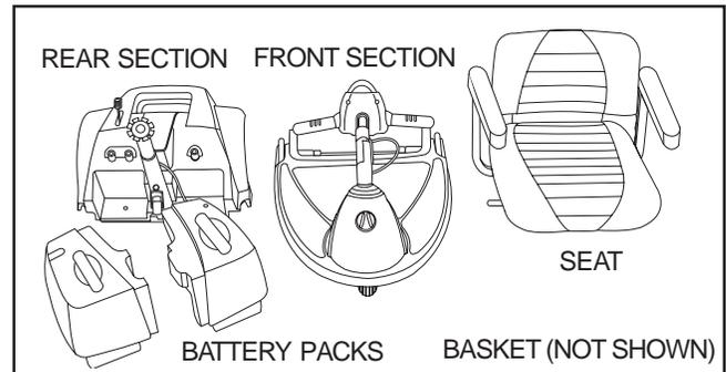
Figure 13. Scooter Components
