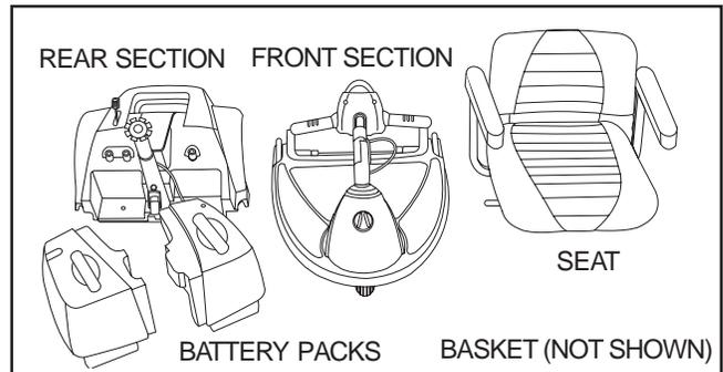
Figure 13. Scooter Components
