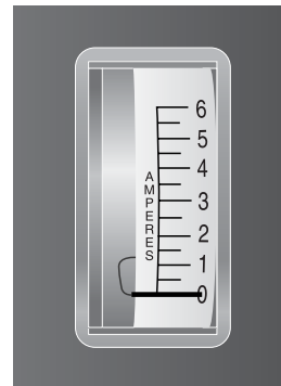
FIGURE 8A. AMMETRE INDICATES BATTERIES ARE FULLY CHARGED
