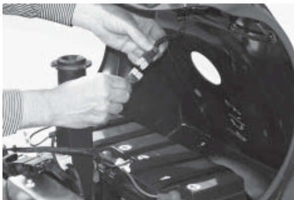
Figure 13. Unplug the Rear Light Harness
