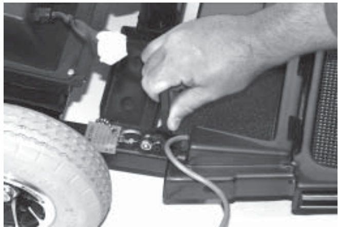
Figure 18. Push Cam Locks Forward
