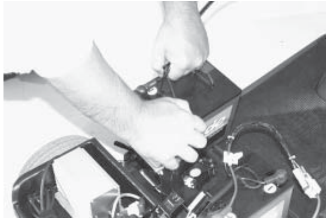
Figure 16. Lift Batteries Off Scooter
