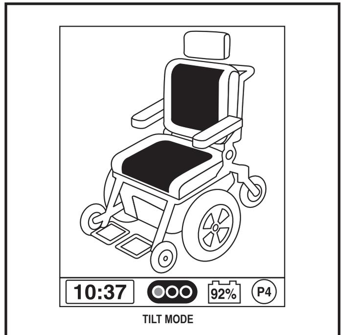
Figure 4. Actuator Mode (Q-Logic)
