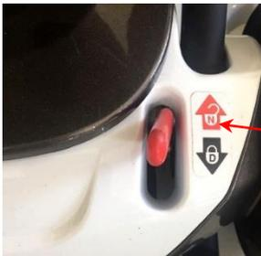
Free- Wheeling Lever/ Maximum required hand-arm force on the lever is 19 N for engaging and 35 N for disengaging
