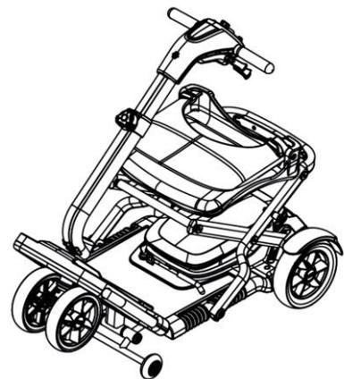
3) Lock the scooter onto the open position by pulling the seat up and pushing the tiller forward until a click sound is heard. Make sure the adjustment knob is locked into position. Insert the key and turn it to power the scooter. Begin using your scooter and enjoy your ride!
