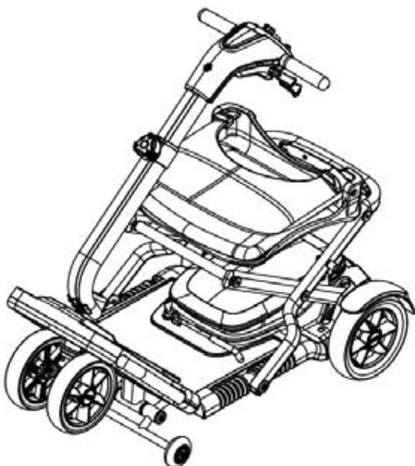
3) Lock the scooter onto the closed position by pushing the tiller down until a lock is heard.
