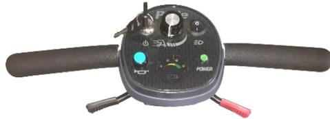
Finger Lever Control/Maximum Force Applied on Lever is 4N
