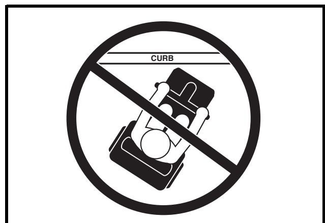
Figure 3A. Incorrect Curb Approach
