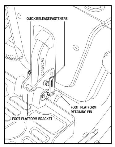
Figure 18. Foot Platform Adjustment
