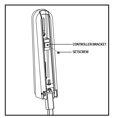
Figure 17. Underside of Armrest
