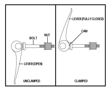
Figure 19. Quick Release Fastener Operation
