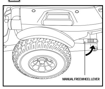
Figure 8. Drive Mode (Drive Engaged)
