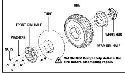
Figure 28. Jazzy 1103 Ultra Drive Wheel Disassembled
