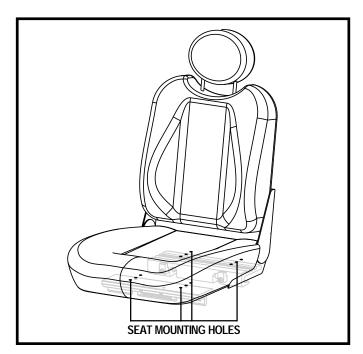
Figure 15. Seat Mounting Holes
