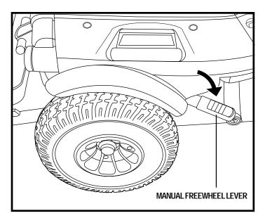
Figure 9. Freewheel Mode (Drive Disengaged)
