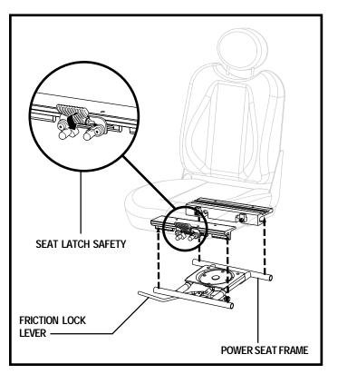
Figure 11. UMS - Power Elevating Seat System
