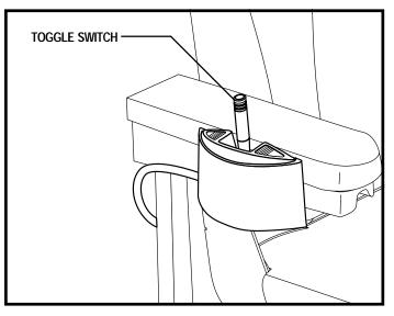
Figure 26. Power Seat Toggle Switch
