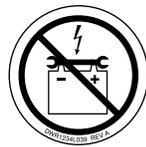
Contact with tools can cause electrical shock.
