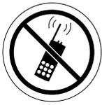
To prevent unintended movement, turn off the power to the electrically-powered mobility vehicle before using a cell phone, two-way radio, lap-top, or any other type of radio transmitter.
