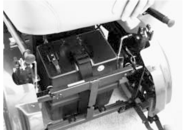
Figure 10. Locking the seat frame
