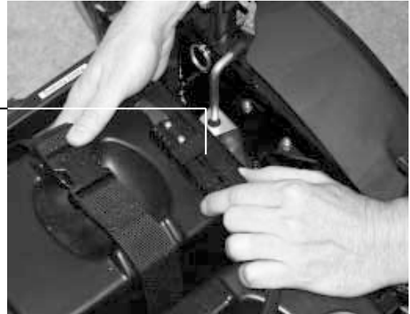
Figure 24. Front to rear battery connector
