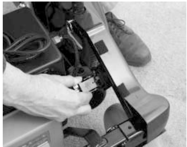
Figure 9. Motor harness connector
