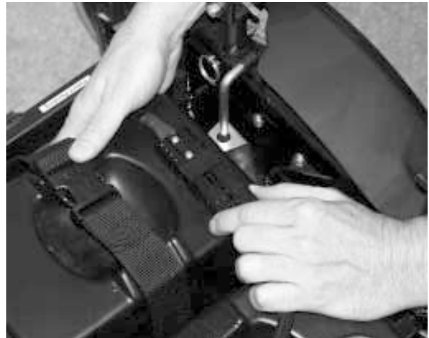
Figure 8. The front-to-rear battery cable connector
