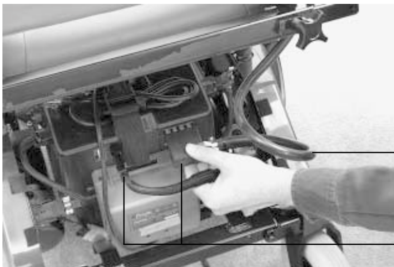
Figure 12. Connecting the controller harness
