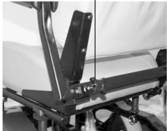
Figure 14. Armrest width adjustment
