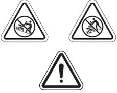
**WARNING! Do not use the power chair while the drive motors are disengaged! Do not disengage the drive motors when the power chair is on an incline or decline, as the unit could roll on its own. Only engage the freewheel mode when on a level surface.**
