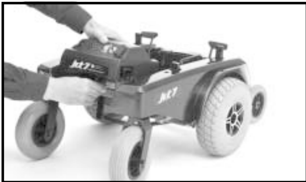
Figure 17. Removing Battery Well Frame
