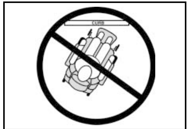
Figure 3. Incorrect Curb Approach
