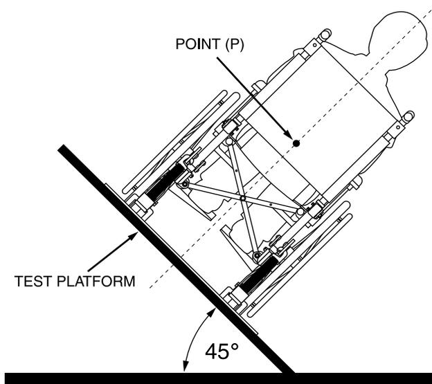
*NOTE: Rear view of the wheelchair and human surrogate secured on test platform and tilted to 45°.*
