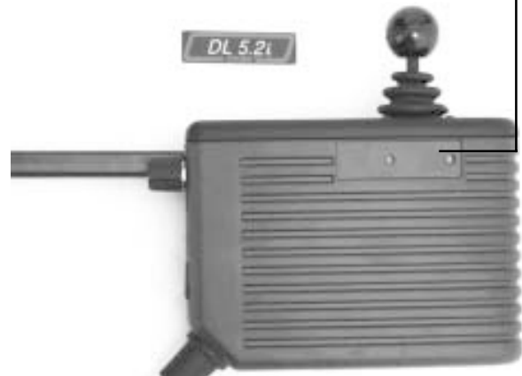
Figure 9. Controller Label Installation
