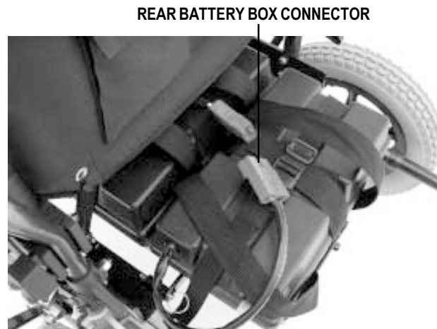
Figure 16. Rear Battery Box
