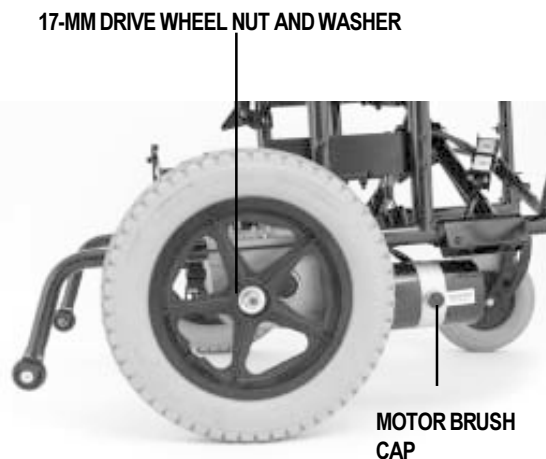
Figure 30. Drive Wheel and Motor Brush Location
