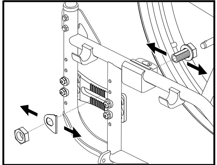
Figure 16. Drive Wheel Position Adjustment
