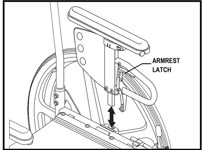
Figure 31 Drop-in Armrest Removal
