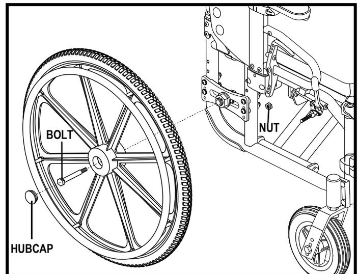
Figure 15. Bolt-on Drive Wheel
