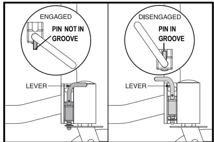
Figure 13. Caster Pin Lock Operation
