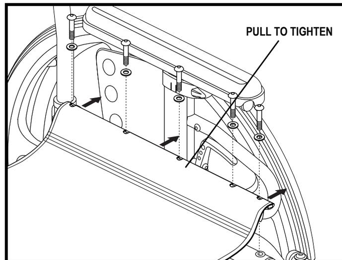
Figure 46. Seat Tension Adjustment
