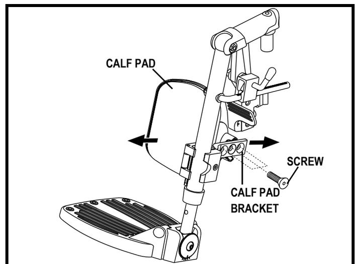
Figure 27. ELR Calf Pad Depth Adjustment
