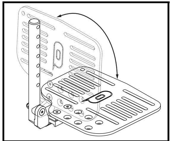
Figure 28. Foot Plate Flip Up Adjustment
