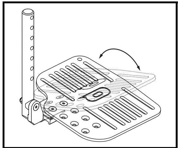
Figure 29. Foot Plate Angle Adjustment
