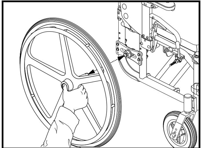
Figure 14. Quick Release Drive Wheel
