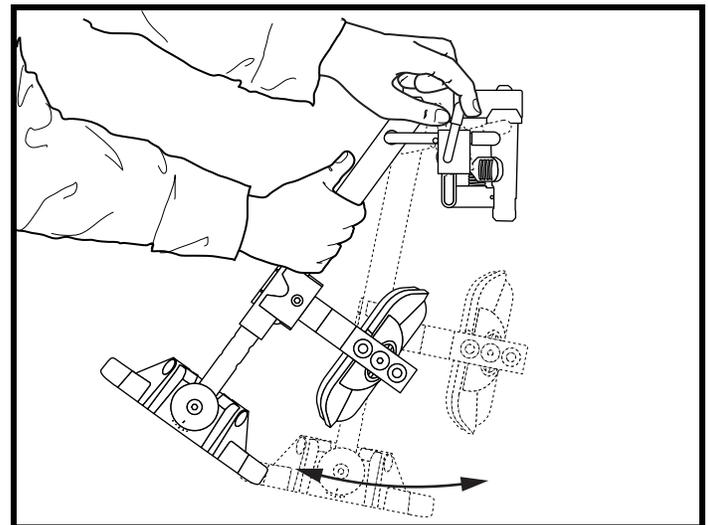
Figure 25. ELR Angle Adjustment
