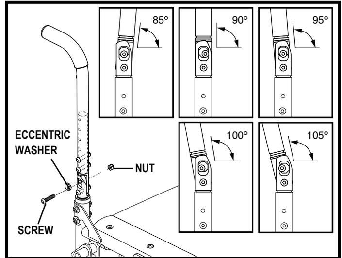
Figure 19. Seatback Angle Adjustment
