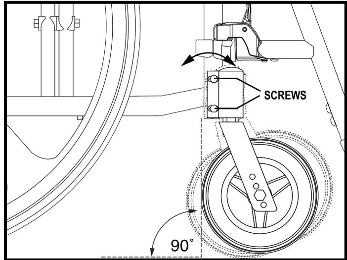
Figure 39. Caster Angle Adjustment
