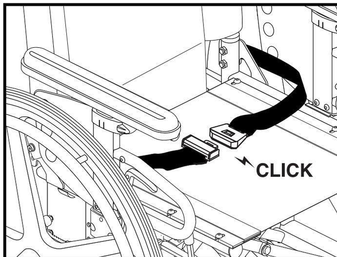
Figure 43. Positioning Belt Adjustment
