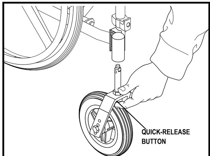
Figure 41. Quick-release Caster Removal
