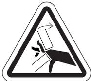
**Pinch/Crush points created during assembly.**
