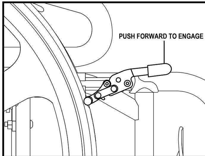
Figure 6. Right Wheel Lock Engaged (Push-to-lock Shown)
