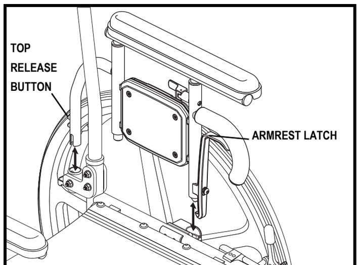
Figure 36. Dual-post Armrest Removal
