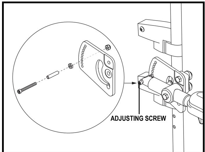
Figure 35. Latching Flip-up Armrest Angle Adjustment
