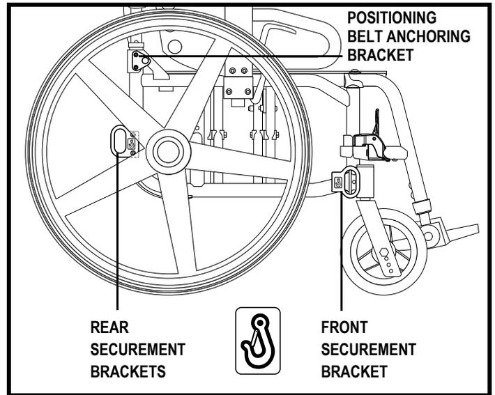
Figure 12. Securement Brackets
