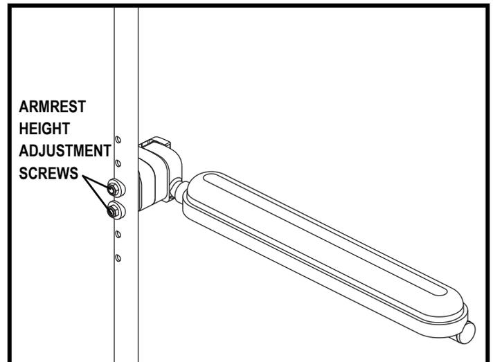
Figure 33. Flip-up Armrest Height Adjustment
