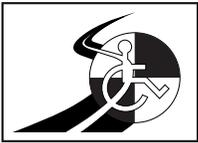
**Indicates that wheelchair, with similarly labeled seating system, conforms to ANSI/RESNA WC/Vol. 4, Section 19/ISO 7176-19 for transport of an occupied wheelchair in a motor vehicle.**
