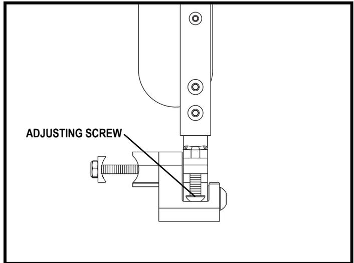
Figure 34. Non-latching Flip-up Armrest Angle Adjustment
