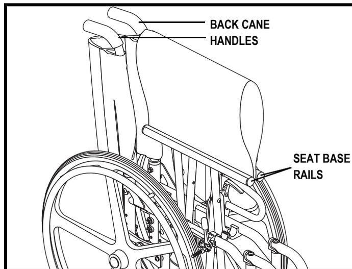
Figure 10. Lifting Points
