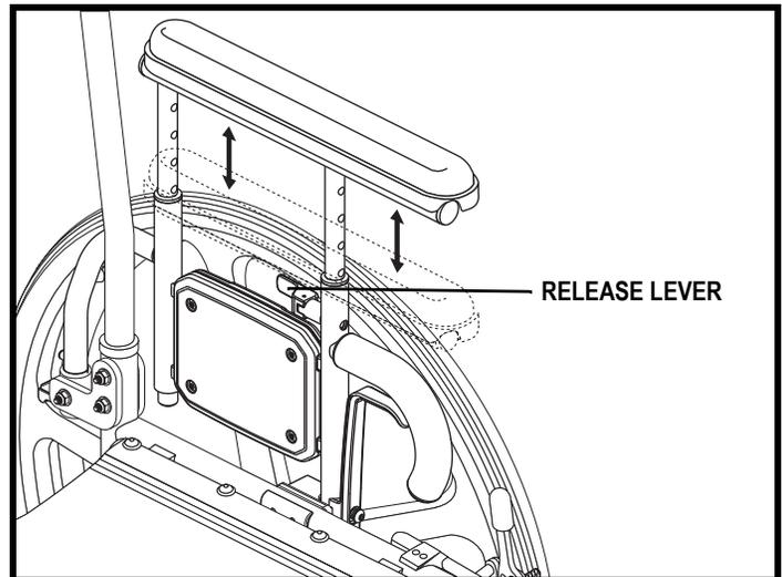
Figure 37. Dual-post Armrest Height Adjustment
