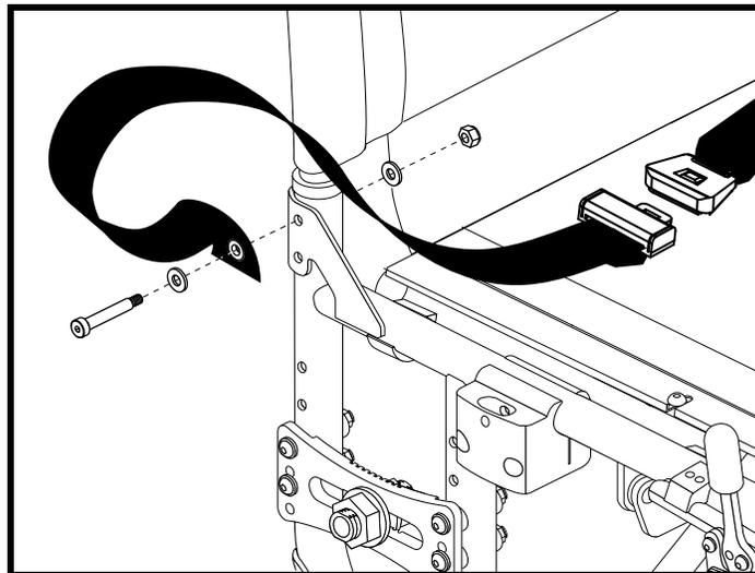
Figure 42. Positioning Belt Installation
