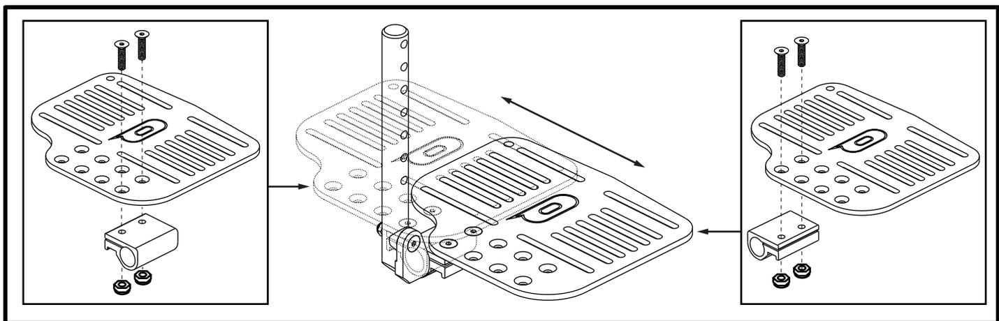
Figure 30. Foot Plate Depth Adjustment
