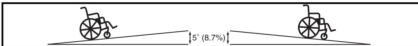
Figure 1. Maximum Safe Slope (Ascending and Descending)
