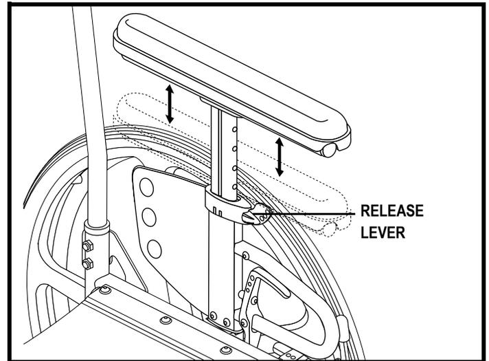
Figure 32. Drop-in Armrest Height Adjustment
