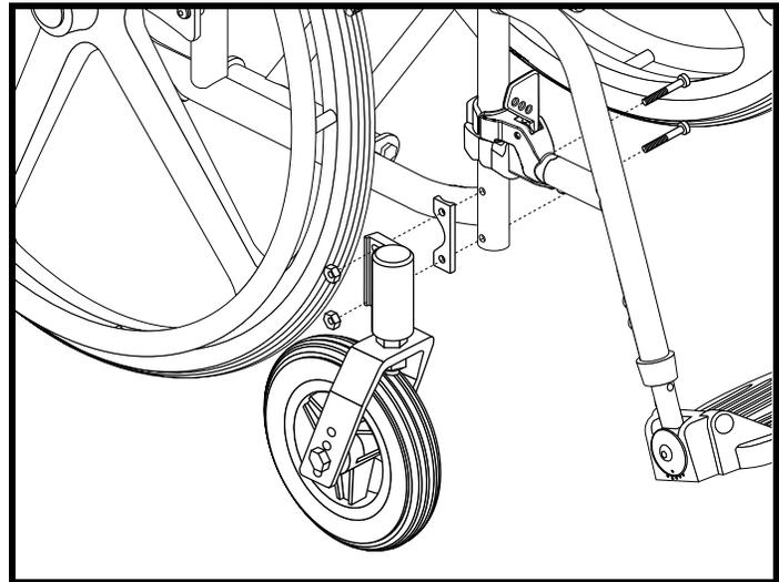
Figure 40. Bolt-on Caster Removal
