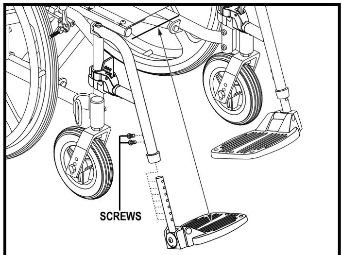
Figure 23. SFR Foot Plate Adjustment
