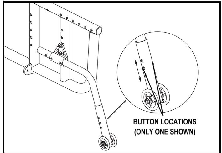
Figure 18. Anti-tip Wheel Adjustment
