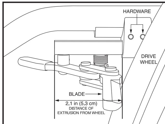
Figure 45. Scissor-style Wheel Lock Adjustment
