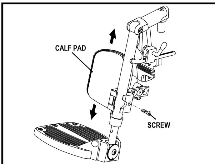
Figure 26. ELR Calf Pad Height Adjustment
