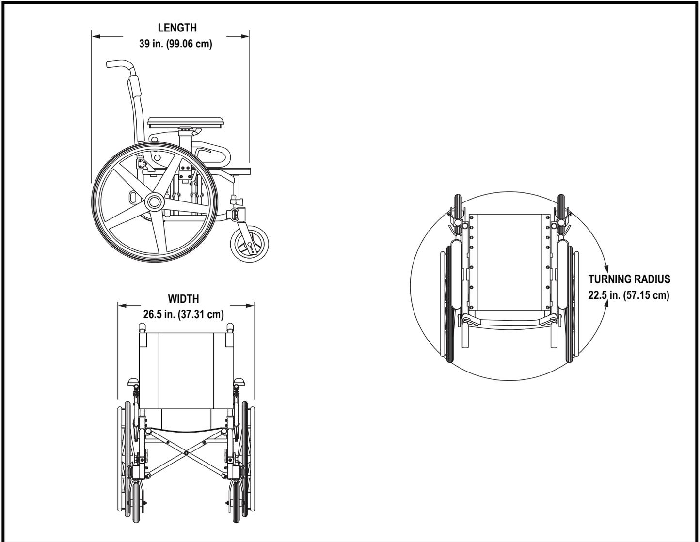
Figure 47. Litestream XF Dimensions and Ground Clearance
