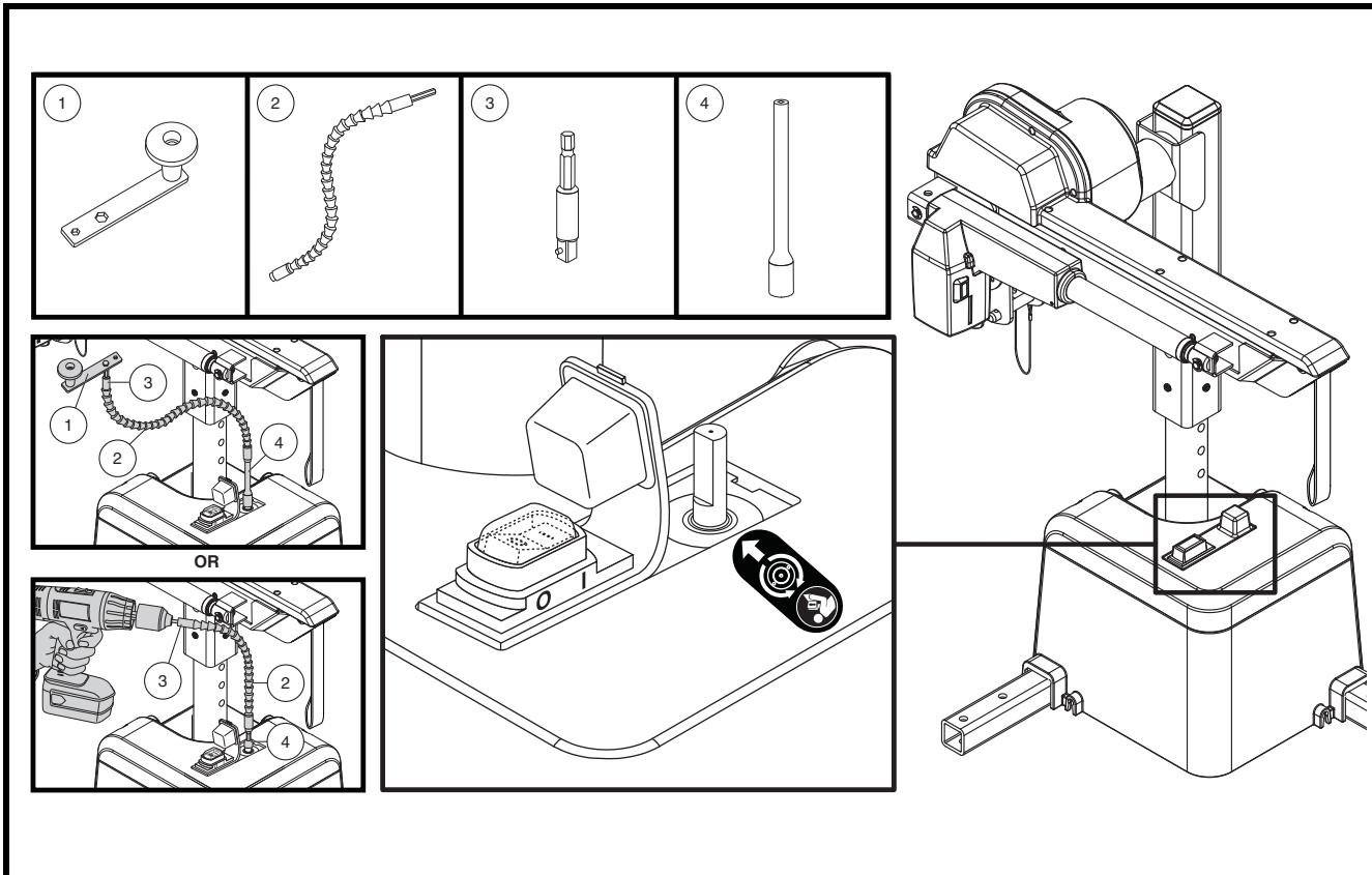
Figure 10. Manual Overide Operation
