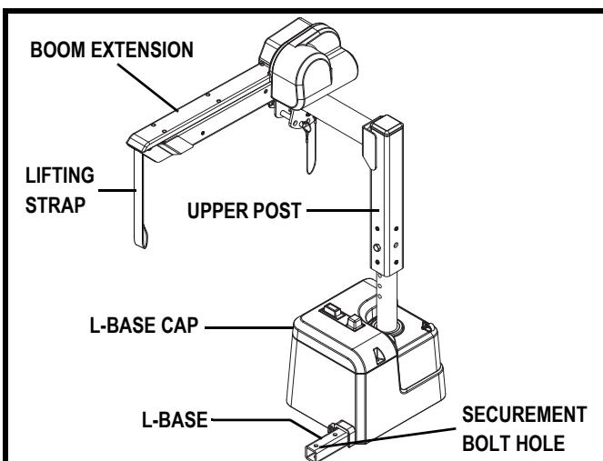
Figure 2. Fully Assembled Lift System
