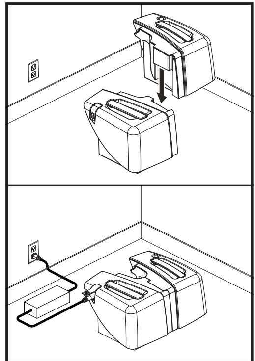
Figure 19. Battery Box Charging (Models 66 and 67)
