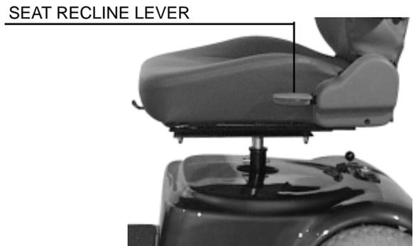
Figure 11. Seatback Adjustment Lever
