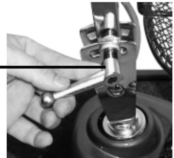
**Figure 8b. Reposition Tiller Adjustment**
