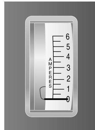
FIGURE 12. AMMETER INDICATES BATTERY IS FULLY CHARGED
