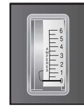
Figure 8. Ammeter Indicates Battery Is Fully Charged
