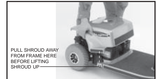
Figure 16. Rear Shroud Removal
