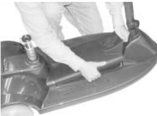
FIGURE 19. LIFTING THE BATTERY/CHARGER PACK
