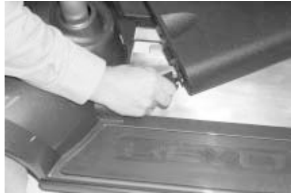
FIGURE 21. WIRING HARNESS REMOVAL/RECONNECT
